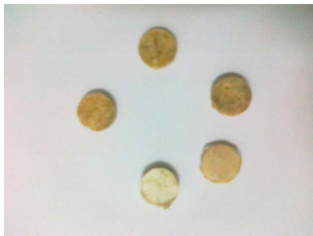
Figure 2. Pellets prepared from the PU–PMMA–TiO 2 blends. [Color figure can be viewed in the online issue, which is available at wileyonlinelibrary.com .]
